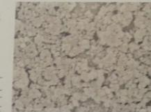
Figure 4: SEM image of the plasma-synthesized powder with Al:Urea molar ratio of 1:4
