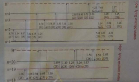
Fig. 4 Flows of electrons for low lying excited states and high lying excited states ( m^{-2} s^{-1} ). The straight arrows denote the non-radiative processes and the dashed arrows represent the radiative processes. The brackets denote the power of 10 by which the number should be multiplied ( \times 1.0 \times 10^{-4} s )
