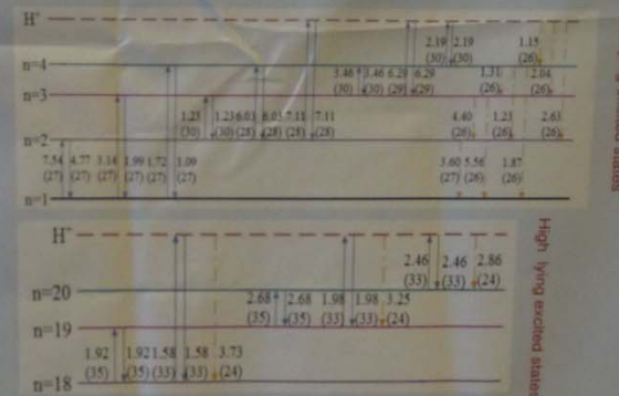
Fig. 3 Flows of electrons for low lying excited states and high lying excited states ( m^{-2} s^{-1} ). The straight-arrows denote the non-radiative processes and the dashed arrows represent the radiative processes. The brackets denote the power of 10 by which the number should be multiplied ( \times 1.0 \times 10^{-4} s )
