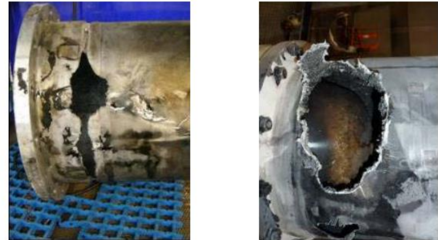
Figure 6-36: Typical views of a HV GIS enclosure in the case of burn-through.
