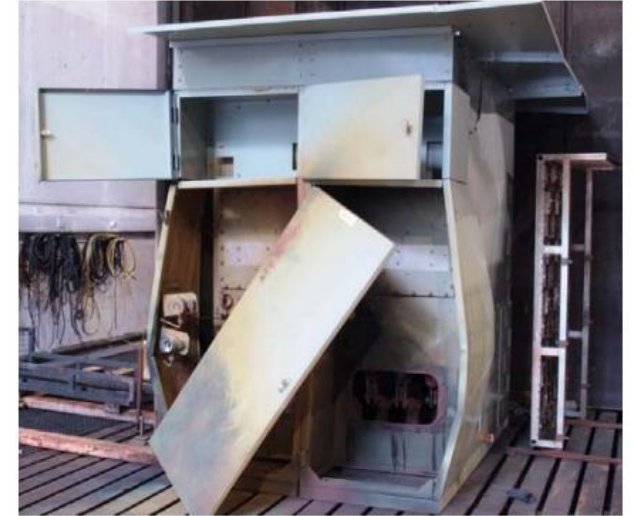
Figure 6-2: Test object after arc resistance test.
