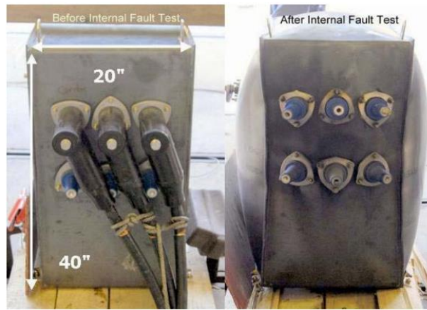
Figure 6-6: Deformation of structure after an internal arc test in the SF 6 -filled switch.
