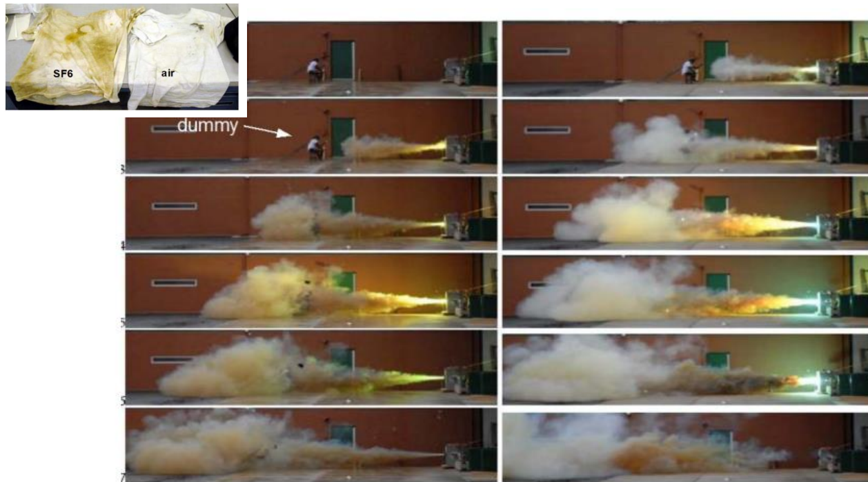
Figure 5-6: Photographic impressions of the release of hot gases as a result of arcing in SF 6 (left column) and air (right column). Arc duration was 1 s, pictures are taken with an interval of 0.2 s.
